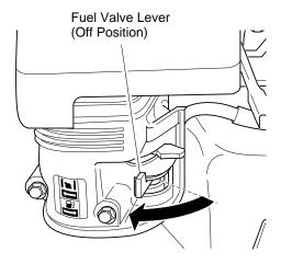
Figure 30 - Fuel Valve Lever Off (Model RGH7500AIE Shown)
